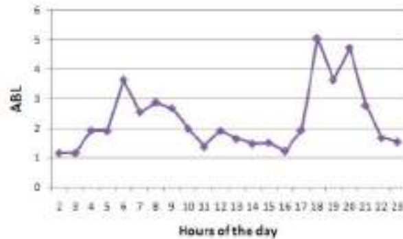
Figure 4.8: Variability of ABL during the day on path B and with 200 messages per second path C that exhibited an average behavior in terms of delay, PLR and ABL.
