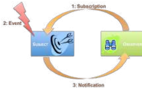
Figure 1.7: Operational schema of a generic event-based architecture
