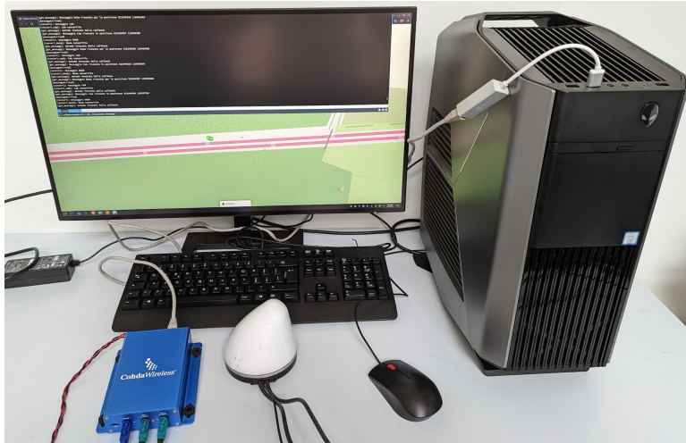
(b) HIL test setup and physical connections. In the bottom half of the picture, in blue, the Cohda MK5 OBU.
