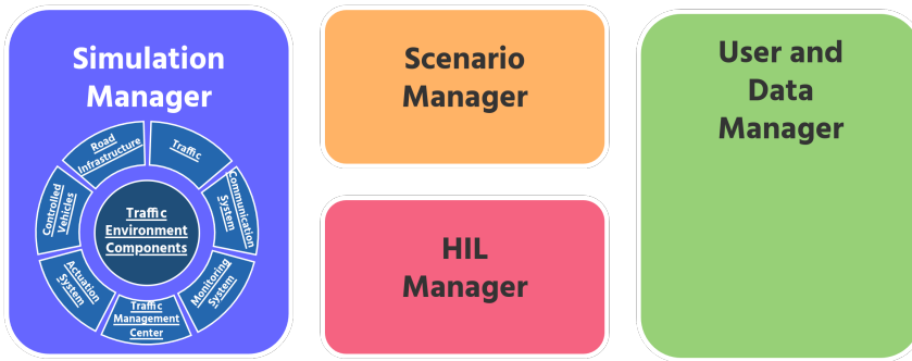
Figure 4.1: High-Level architecture for the co-simulation platform
