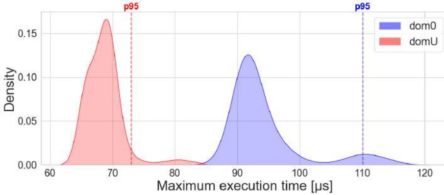
Figure 3.10: Distribution of maximum execution times for voter( dom0 ) and replica( domU ) by fixing host-level scheduler factor to null level, the CPU affinity factor to the One-to-One level, and the stress factor to CPU .
