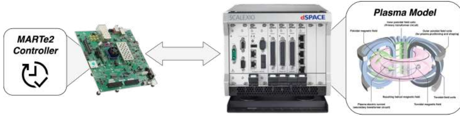
Figure 5.11: Hardware-in-the-loop Simulation Setup
